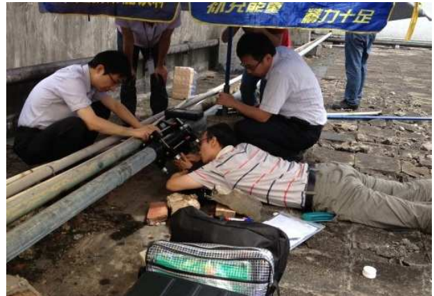
07.2013 Non-invasive supersonic measurement for air compressor pipes- an energy saving improvement project.
